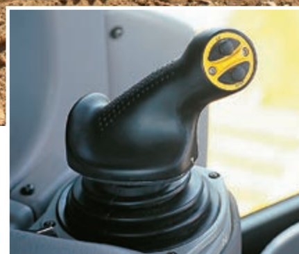
Comandi palmari PCCS (Palm Command Control System)
