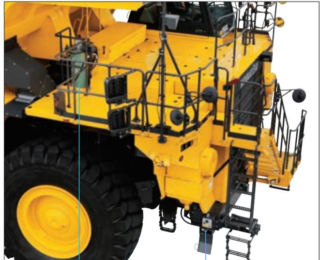
Grease pump pump and reservoir    Refill port
